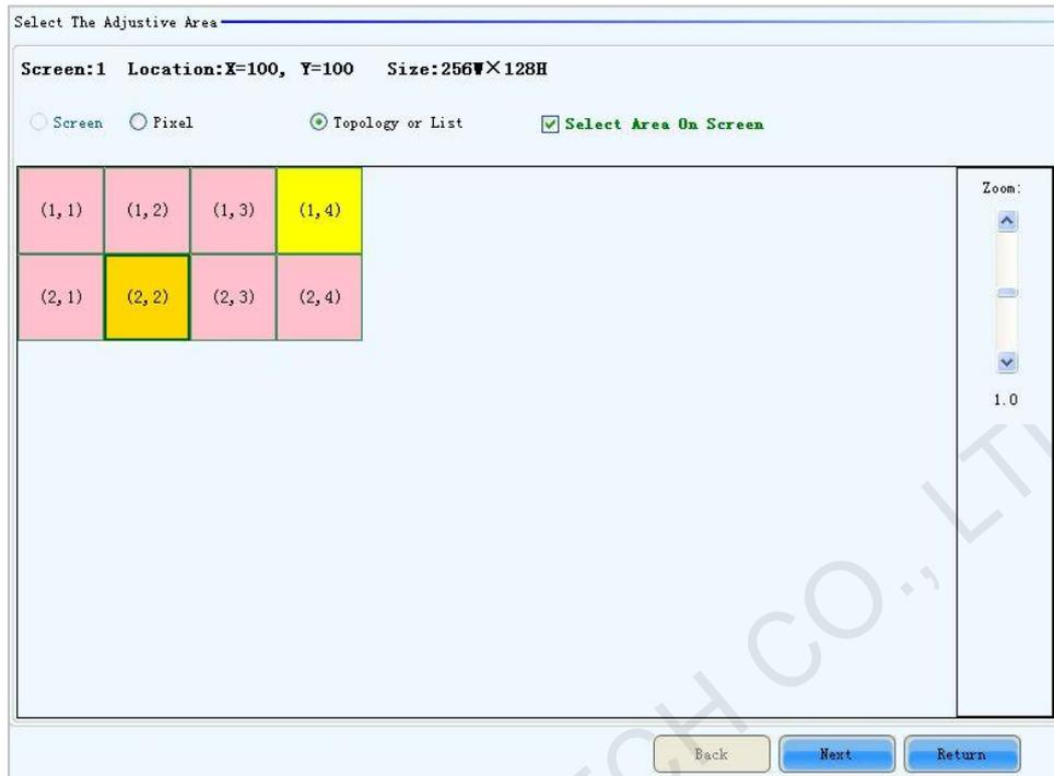
Step 2 Select the adjustment type. If Adjust Own Effect option is selected, the color adjustment of selected area is independent to the other areas of the LED display. If **Effect As Other Selected Area** option is selected, the color of the selected area will be adjusted according to the reference area color. The selected area color will look similar to the reference area color after the adjustment operation.
